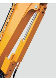
The standard boom cylinder cover and dozer cylinder cover provide additional protection.
