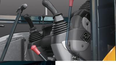
The left-side console can be tilted, making it easier to enter and exit the cabin.
